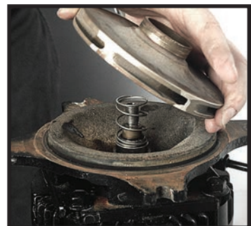
Aligning impeller and spring Figure 5.1L
