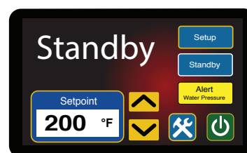
Yellow Alert Icon showing Water Pressure Fault
